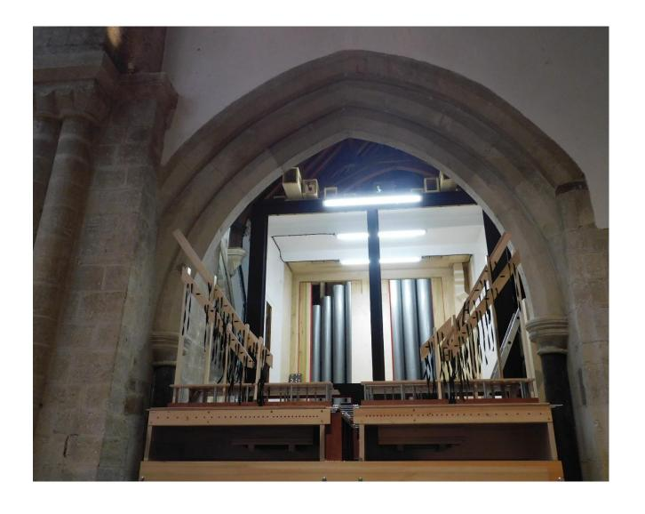
Pipes installed in the Swell Box.
